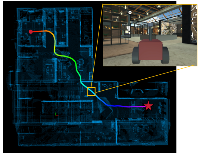
Fig. 8: Unity-Based Simulation of H-PAMO*.
